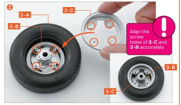
Hold **3-B** in place and turn the tyre over. Align the **Inner Rim 3-C**, which forms the inside of the wheel, with the four screw holes on **3-B** as shown, and fit it into place.
